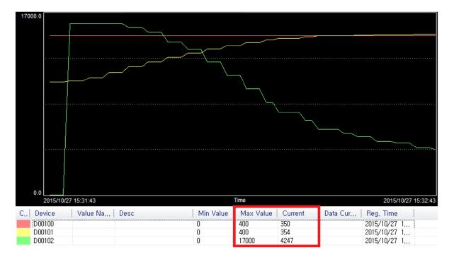
Through the Trend function, it is possible to check the status of the SV (Set Value), PV (Process Value), and MV (Manipulation Value).
