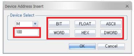
\*If the last address of the Bit device does NOT end with 0, only BIT type can be selected.
