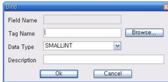
This is used to set up the tag linked with the run result of a SQL or the contents of a statement.
