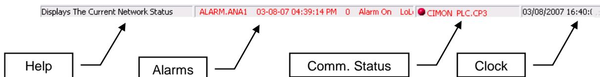
**Help** This is used to show the brief description about a corresponding menu when the mouse is put on a menu or a toolbar.
