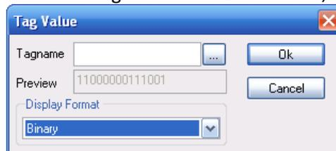
3. “Binary Number” is added and displayed in the Format. Here, if you enter a tag name and click the menu to run the CimonX, the corresponding tag value will be displayed in binary number.
