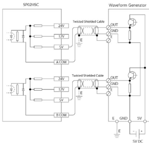
2. When waveform generator outputs 24 V PNP open collector output. (CM3-SP02HSC)
