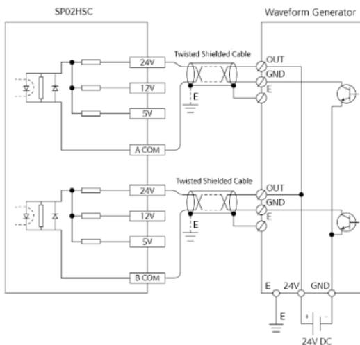
4. When waveform generator outputs totem pole output (voltage type). (CM3-SP02HSC)
