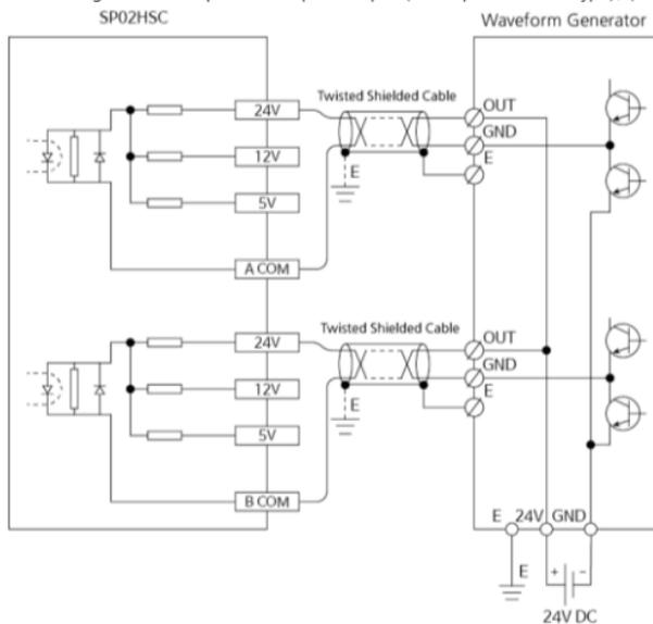
6. When waveform generator outputs line driver output. (CM3-SP02HSD)
